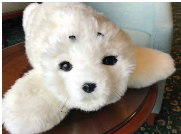
The PARO robot resembles a furry baby seal. Using sensors to perceive people and its environment, it can squeal, blink and turn its head in response to touch, light, sound, temperature and positioning. Photo: Sharon Stoddart
